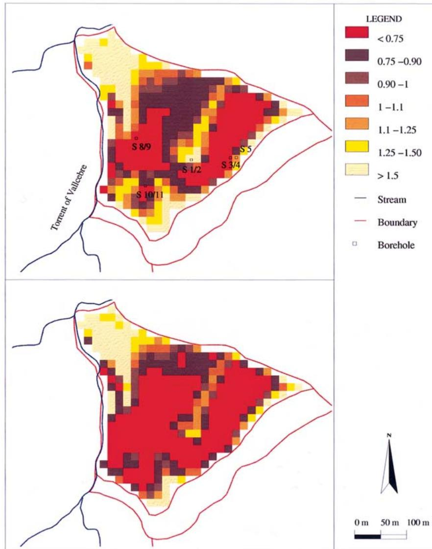
Figure 5. Map of factors of safety at each cell of the Vallcebre landslide. The analysis has been performed considering a friction angle of  $8^\circ$  and both low groundwater (top) and high groundwater levels (bottom).
