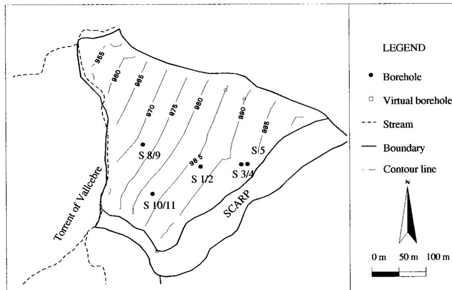
Figure 4. Groundwater level of the lower unit of the Vallcebre landslide generated by interpolation from available piezometers and with the inclusion of a seepage front at the landslide foot. The surface corresponds to the highest groundwater level recorded in the piezometers (January, 1997).
