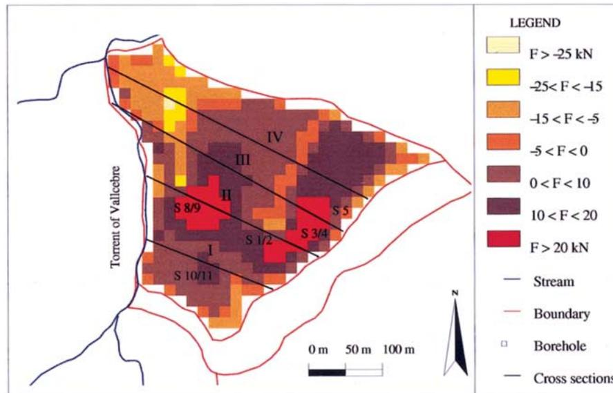
Figure 6. Map of resultant sliding force (in kN) at each cell of the Vallcebre landslide for the highest recorded water levels.
