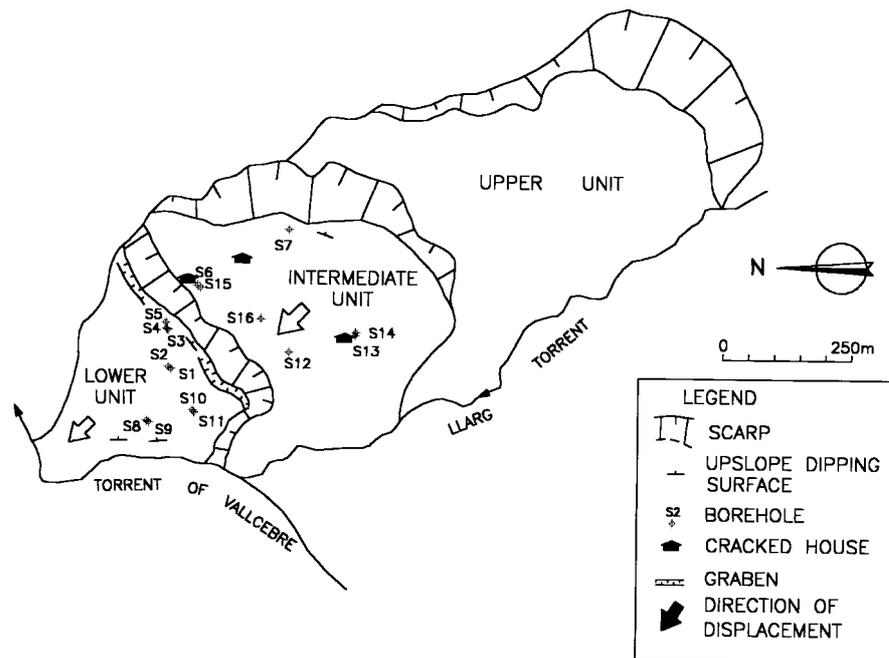
Figure 1. Geomorphological sketch of the Vallcebre landslide. The location of boreholes is also shown.
