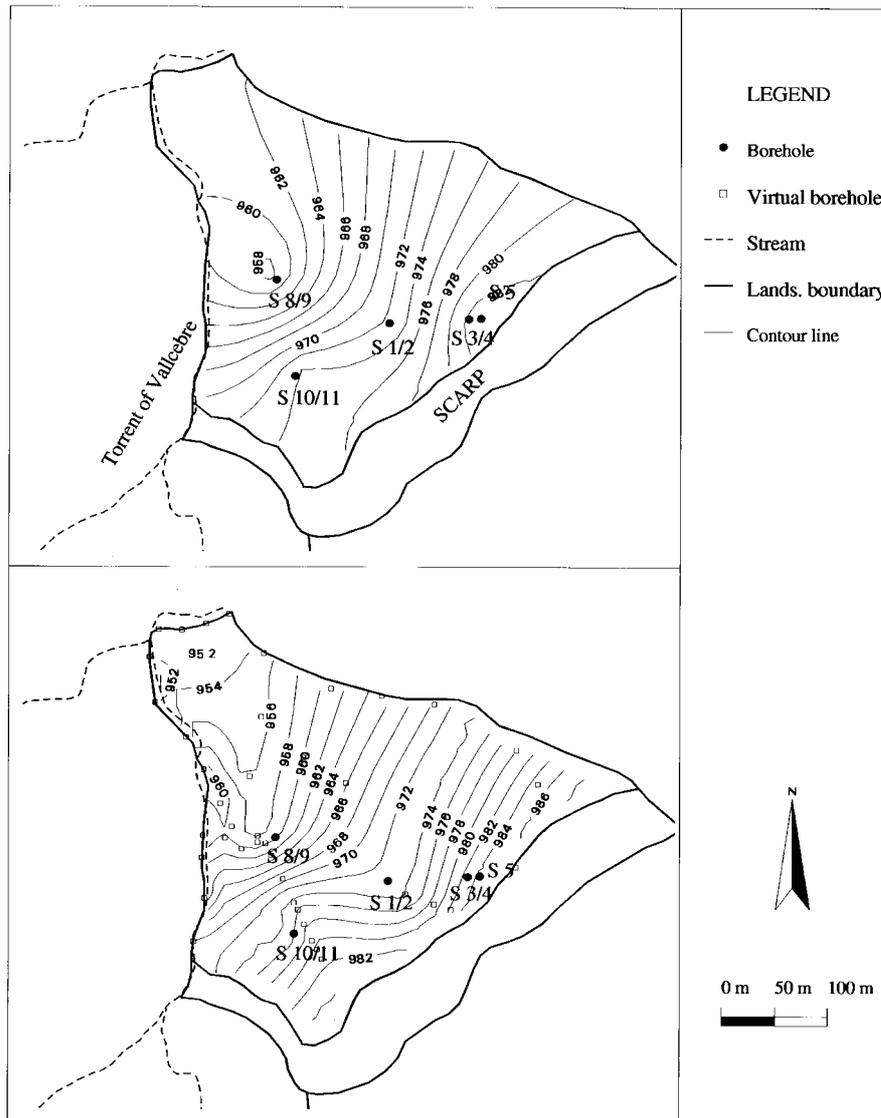
Figure 3. Surface of rupture of the lower unit of the Vallcebre landslide generated by interpolation from available inclinometers (top). The same surface generated after the inclusion of virtual boreholes (bottom).
